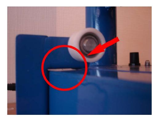
**C.** Unsettle the lower plate with the fixation screw then unsettle the base « U » thanks to an "allène" key. Then, settle on the double post trolley:
