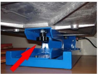
A. When the plate of origin is removed, put the new plate on the press. The central opening situated on the base is kept for the screw of fixation. The two other central opening are intended for the nipple (head of screw fixed under the plate) which comes to ensure a good maintenance of the plate. Place this nipple on the up opening or the left one according to the orientation of the plate that you need.
